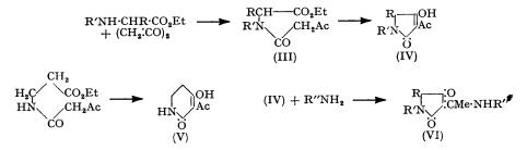
palladium on charcoal catalyst. However (IV; R = Me, R' = H) and (IV; R = H, R' = Ph) resisted hydrogenation under these conditions which, in confirmation of the work of Clutterbuck *et al.* (*loc. cit.*), were found adequate for the reduction of  $\alpha$ -acetyl-tetronic acids. The bromination of  $\alpha$ -acetyltetramic acids did not proceed analogously to that of  $\alpha$ -acetyltetronic acids (Clutterbuck *et al.*, *loc. cit.*) (cf. Part IV), but gave only intractable products.
